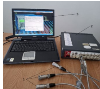
Fig. 1 Elements of the measuring chain: 1 – accelerometers, 2 – NetdB12, 3 – computer with appropriate software
