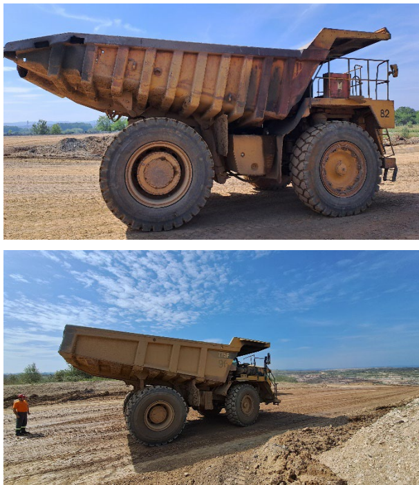
Fig. 2 Caterpillar dumpers: CAT 777C and CAT 775F
